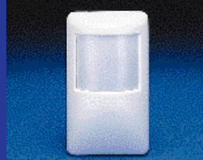
Passive Infrared detector "sees" an intruder's body heat.
