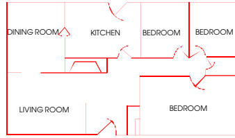
A smoke detector shall be located between the sleeping area and the rest of the house. - Refer to N.F.P.A. #74 Appendix B-1.1 thru B-10.
